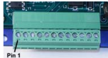
P1 Connector – Pin 1 Location
